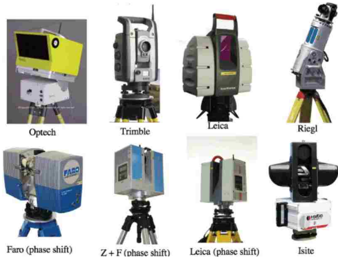
Figure 1.1: Ground-based LiDAR scanners (time-of-flight unless noted as otherwise) [8, 9, 10, 11, 12, 13, 14, 15, 16].
