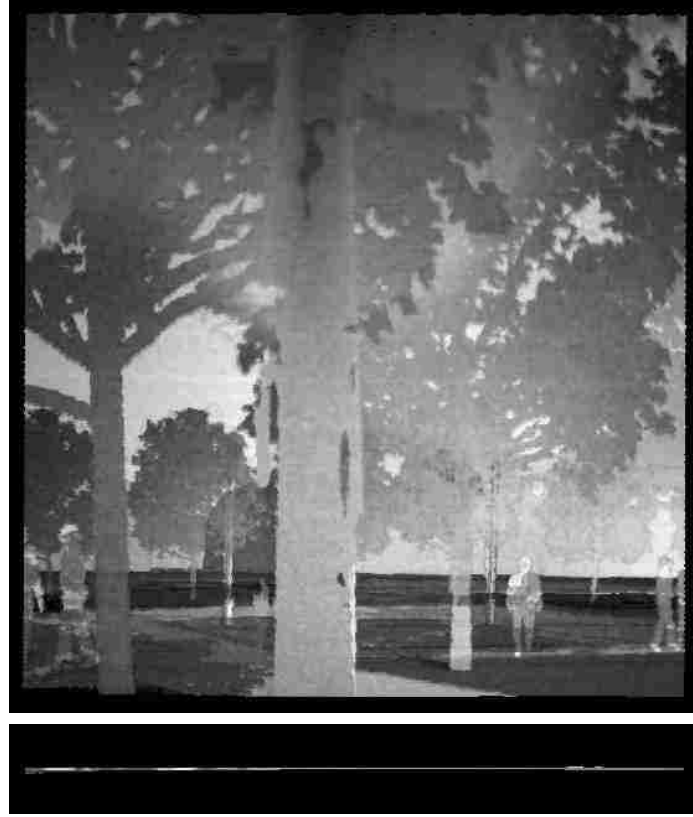
Figure 3.12: The 3-D reconstruction of a flat board with intensity texture, through 4 pattern, 16 period PCPS using hybrid decoding method showing the (top) front and (bottom) top view.
